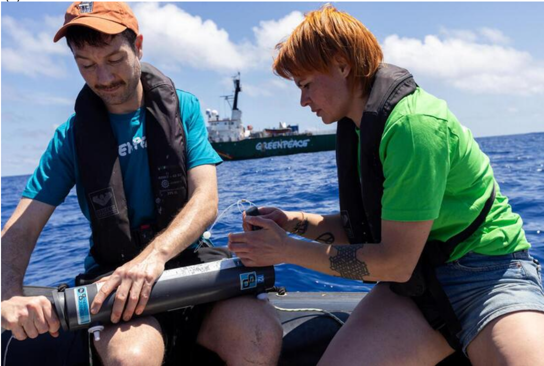
Figure 3. eDNA water sampling being conducted by handheld niskin aboard (a) the Arctic Sunrise and (b) an inflatable RHIB.
