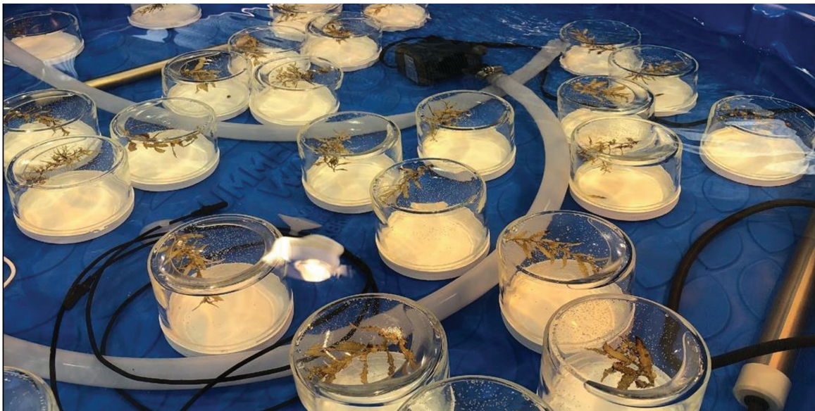
FIGURE 2.5. Growth and environmental tolerance experimental setup in the Eckerd College greenhouse. Individual Sargassum specimens in glass jars containing salinity treatment were submerged in circulating water baths with regulated temperatures. Photo credit: J. Schell.
