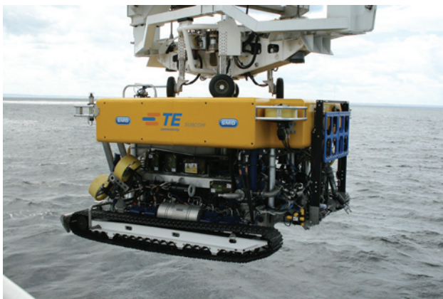
Figure 7.4 SMD remotely operated vehicle with manipulating arms and other equipment for cable repairs and burial (right) and positioning propellers (left). (Photograph courtesy of TE SubCom)
