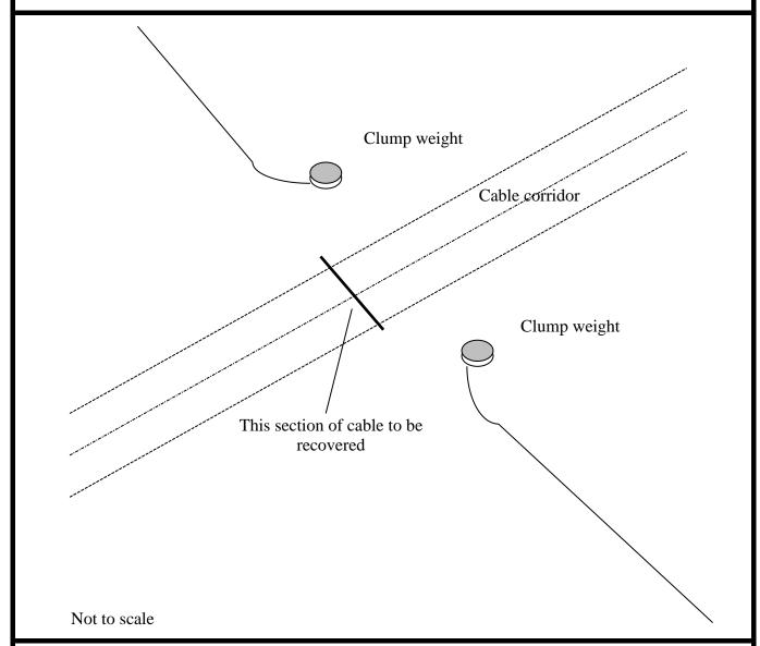
The clump weights shall be concrete discs, typically 0.5 metres diameter by 0.2 metres thick, or other thin sectioned weights, alternatively chain may be used. The object of the weight is to minimise risk of fastening to fishing gear.
