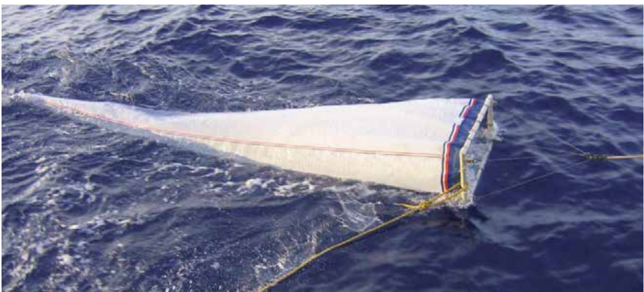
FIGURE 1. Surface skimming neuston net (1 m x 0.5 m) equipped with 333 \mu\text{m} mesh. All tows approximately 1 nm in length while the vessel was sailing at 2 kts.
